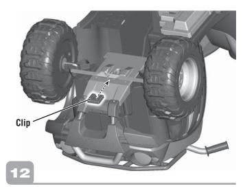
• Slide the clip (open side down) **under** the end of the steering column, as shown.
